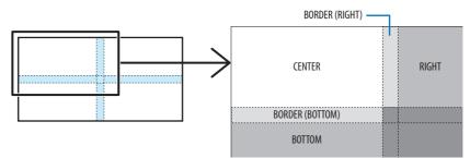
Select the location to adjust from the dropdown list and adjust the Black Level with the Reference, Red, Green and Blue adjustment bars. Select Reset to delete the adjustment value.
