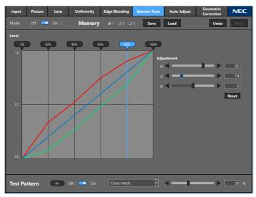
Adjust the intermediate tone colors between projectors. Select the target projector to adjust from the Projector List.
