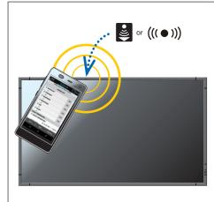
To read/write an adjustment value/setting value of the display, bring the terminal close to the Intelligent Wireless Data sensor of the display and press the READ / WRITE button of the application. Or, after pressing the READ/WRITE button of the application, bring the terminal close to the Intelligent Wireless Data sensor of the display.
