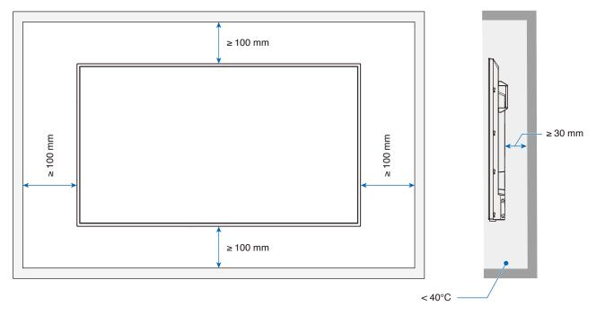
**NOTE:** The maximum environmental operating temperature of the monitor is 40°C. This monitor has internal temperature sensors.
