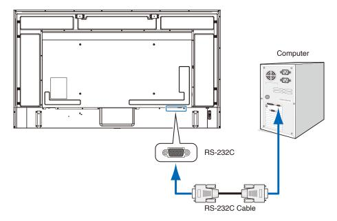
NOTE: • If your computer is equipped only with a 25-pin serial port connector, a 25-pin serial port adapter is required.
