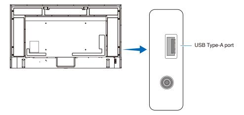
NOTE: • Check the connector shape and orientation when connecting the USB device or cable.
