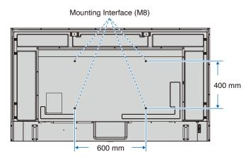
Mounting accessories can be attached with the monitor in the face down position. To avoid scratching the LCD panel, always place a soft cloth, such as a blanket that is larger than the monitor's screen area, on the table before laying the monitor face down. Make sure there is nothing on the table that can damage the monitor.
