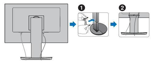
**NOTE:** Please check that you can still rotate, raise and lower the monitor screen after you have installed the cables.
