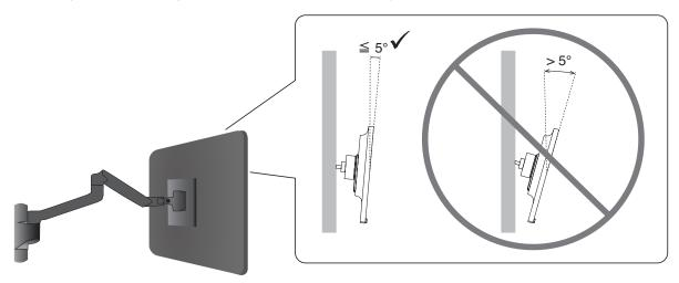
· After mounting, please carefully ensure the monitor is secure, and not able to come loose from the wall or mount.
