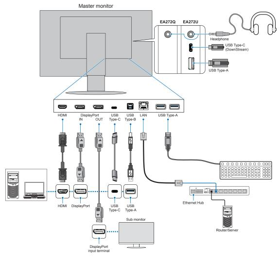
To maintain compliance with EMC regulations, use shielded cables to connect to the following terminals: USB port, USB Type-C port, HDMI input terminal and DisplayPort input terminal.
