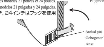
The bottom hook is used for 26" displays.
