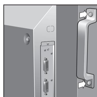
Secure the handle by 2 screws (Screw-A).
