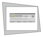
TIP: If you are adjusting [KEYSTONE], [CORNERSTONE] will not be available. If this happens, press and hold the 3D REFORM button for a minimum of 2 seconds to reset the [KEYSTONE] adjustments.
