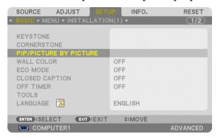
The [PIP/PICTURE BY PICTURE] menu item has the following three options: MODE, POSITION, and SOURCE. Use the ▲ or ▼ button to select [MODE], [POSITION] or [SOURCE] and press the ENTER button.
