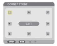
This option allows you to correct trapezoidal distortion. Selecting this item will display the Cornerstone adjustment screen. ( $\rightarrow$  page 40)
