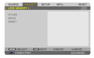
This function serves to store the adjusted values for each input signal when using the LENS SHIFT, ZOOM and FO-CUS buttons of the projector. Adjusted values can be applied to the signal you selected. This will eliminate the need to adjust lens shift, focus, and zoom at the time of source selection.
