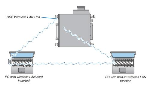
To enable direct communication (i.e., peer-to-peer) between computers and projectors, you need to select the Ad Hoc mode. ( $\rightarrow$  page 149)
