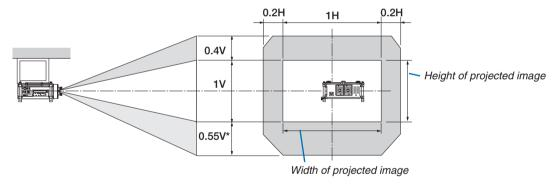
\* The maximum adjustable range for lens shift (V) is 0.5V when the NP32ZL lens is used.
