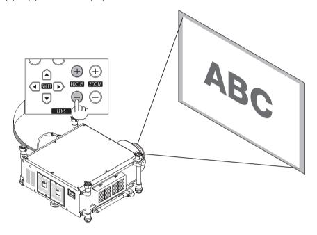
TIP: To obtain the best focus, perform the following (for fixed installation) Preparation: Warm up the projector for one hour.
