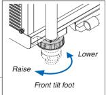
4. Rotate each of the tilt feet to adjust the height while keeping the projector level with the floor/ceiling and perpendicular to the screen when viewed from the side.
