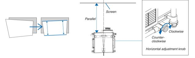
3. Rotate the two front tilt feet to adjust the height to keep the projector level so that the top edge of the screen is parallel with the top edge of the projected image.
