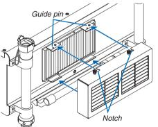
(2) Slide the filter cover to the right and tighten each of the two knobs by turning them clockwise.
