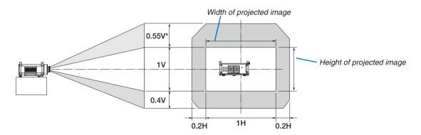
\* The maximum adjustable range for lens shift (V) is 0.5V when the NP32ZL lens is used.
