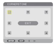
This option allows you to correct trapezoidal distortion. Selecting this item will display the Cornerstone adjustment screen. (→ page 41)
