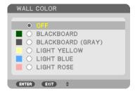
This function allows for quick adaptive color correction in applications where the screen material is not white.
