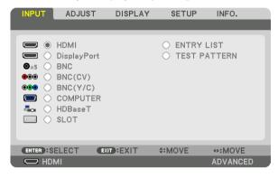
Press the ▼/▲ buttons to match the target input terminal and then press the ENTER button to switch the input. To delete the menu display in the [INPUT] screen, press the MENU or EXIT button.
