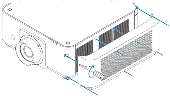
\* If using in normal horizontal orientation, make sure to remove the safety cover.
