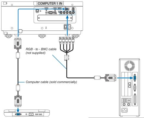
NOTE: Please check the operating manual of the computer as the name, position and direction of the terminal may differ depending on the computer.
