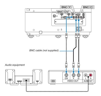
• Select the source name for its appropriate input terminal after turning on the projector.
