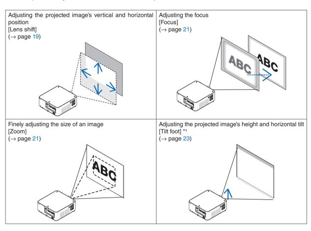
NOTE\*1: Adjust the projected image's height using the tilt feet when you want to project the image at a position higher than the lens shift adjustment range.
