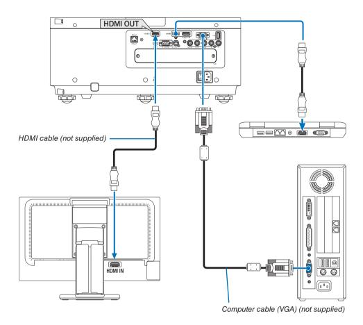
You can connect a separate, external monitor to your projector to simultaneously view on a monitor the computer analog image you're projecting.
