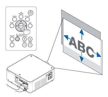
Returning the lens shift position to the home position Press and hold the LENS SHIFT/HOME POSITION button for 2 seconds to return the lens shift position to the home position (nearly center position)
