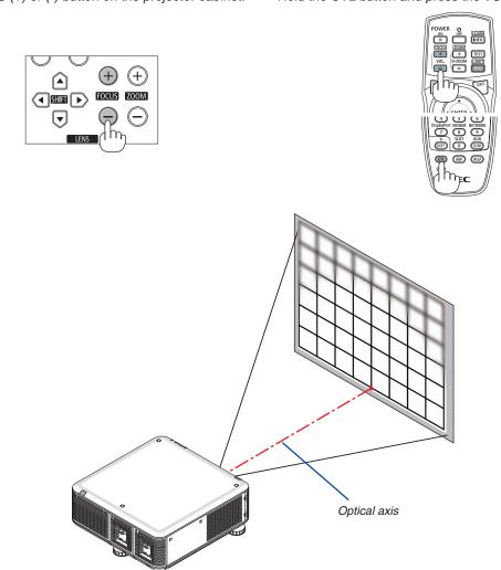
\* With the lens shift in the center position the optical axis is at the center of the image. In this case, adjust the focus at the center of the projected image.
