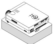
If necessary, adjust the front or rear feet to properly position the projected image on the screen.
