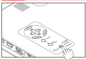
**NOTE:** To turn off the projector, press and hold the Power (ON/STAND BY) button for a minimum of two seconds.
