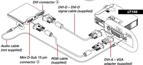
Connection Option 1 when using DVI output Connection Option 2 when using mini D-Sub 15 pin output
