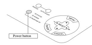
**NOTE:** To turn off the projector, press and hold the POWER button for a minimum of two seconds.
