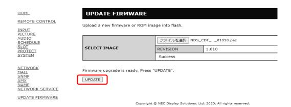
After update has started, "Processing..." message and the progress of the update will be displayed. Also, the LED of this device blinks green.
