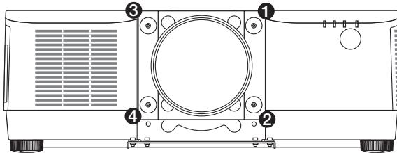
③ Tighten the top 2 adjustment bolts by a quarter turn each time.
