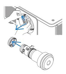
3. Hold the lens unit aligning the labelled arrow on the unit coming top and insert the unit to the projector.
