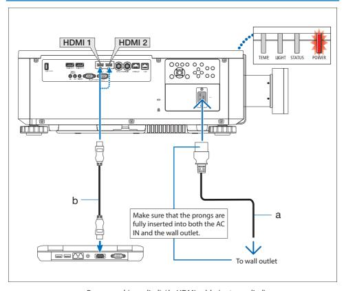
a: Power cord (supplied) / b: HDMI cable (not supplied)
