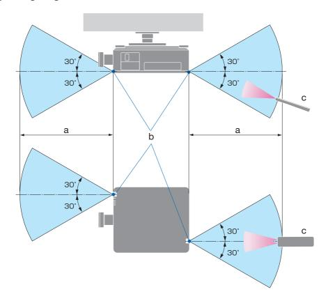
a: 7 m/276" / b: Remote sensor on projector cabinet / c: Remote control
