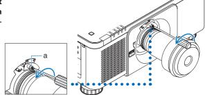
While pressing the LENS release button on the projector's front panel fully in, turn the lens counterclockwise.
