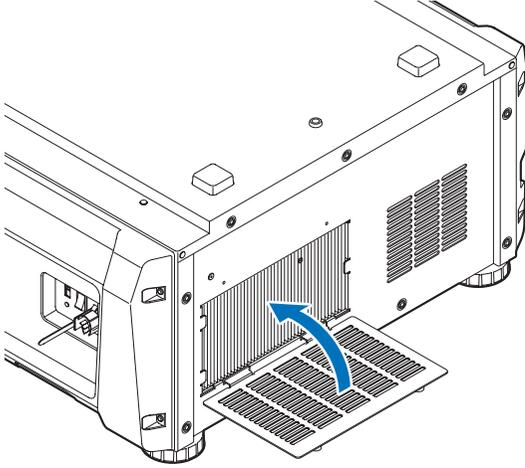
2. Tighten the two knobs clockwise to secure the filter cover.
