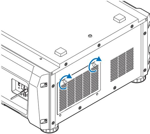
This completes replacing the rear air filter. Next, replace the side air filter.
