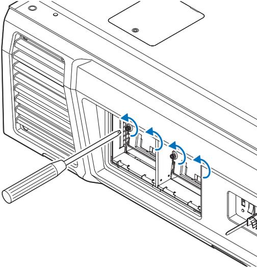
2. Grasp the handle and remove the lamp housing.
