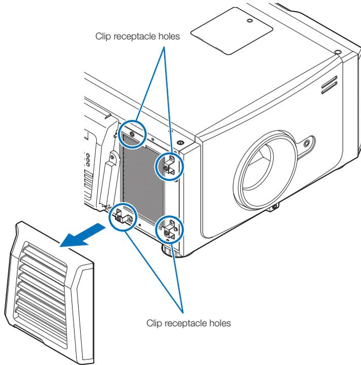
**NOTE** When removing the filter cover, remove it by applying force evenly. If you only apply force to one side, it may cause the clips to become damaged.
