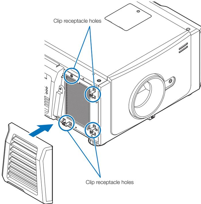
This completes replacing the side air filter. If you have not yet finished replacing the rear air filter, replace the rear air filter next (See page 58).
