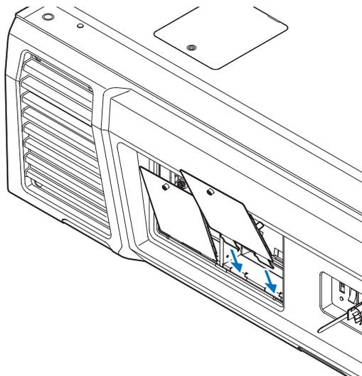
2. Tighten the screw to secure the lamp cover.
