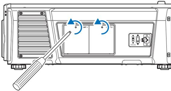
2. Grasp the standoff pillar of the screw securing the lamp cover and pull it up towards you to remove the lamp cover.
